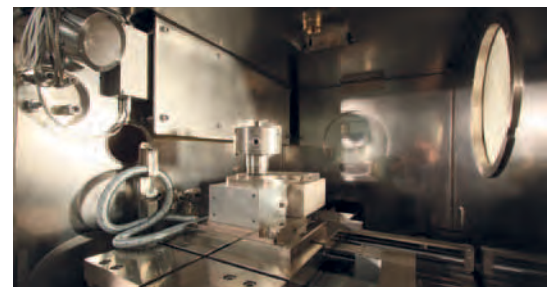
The view into a flexible chamber system with all of the technical options including fast beam deflection.
